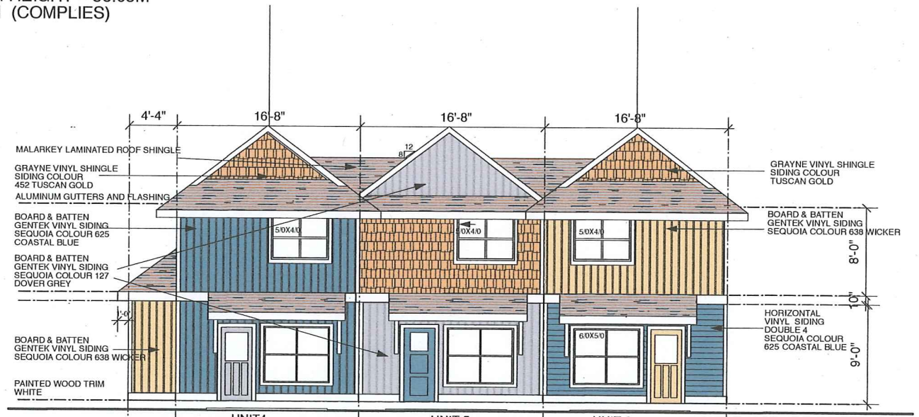
ELEVATION - REAR ENTRY FROM COURTYARD
